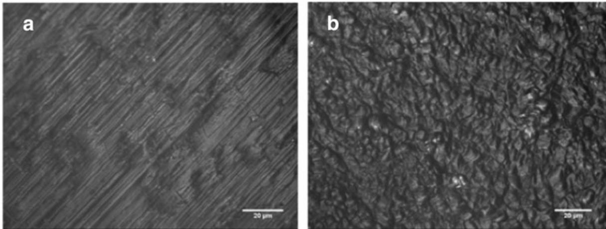
**Figure 1.** Machine-polished (a) versus sandblasted and acid-etched (b) titanium surfaces assessed using scanning electron microscopy. Images are representative of multiple samples from at least five independent preparations. Scale bars are 20 µm.
